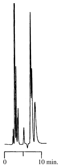
Fig. 7. Chromatogram showing the enantioresolution of DNP-Leu-Ala on SN- \beta -CD bonded phase using the acetonitrile-based mobile phase of 480 ACN/20 MeOH/1 HOAC/2 TEA by volume, (v/v). Note that the retention scale is relatively small. The middle two peaks appear to be a pair of enantiomers based on the results of altering the detection wavelength
